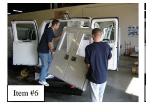
Place **Rear Bulkhead Doorframe** into vehicle
